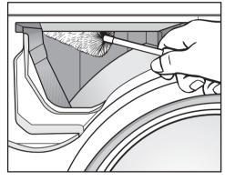
Use a bottle brush to remove any detergent residue and lime deposits from the jets inside the detergent drawer.
